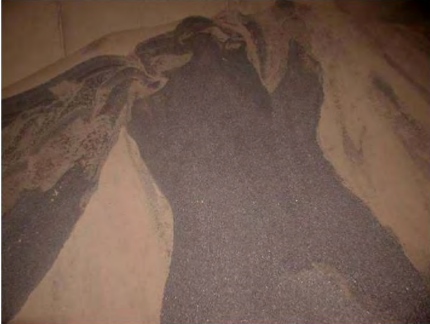
Reactor Accumulation of Unburned Carbon
