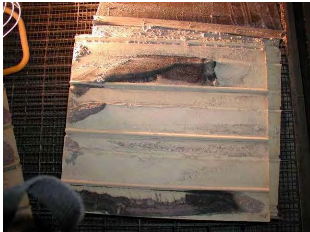
Plate Catalyst With Accumulated Unburned Carbon
