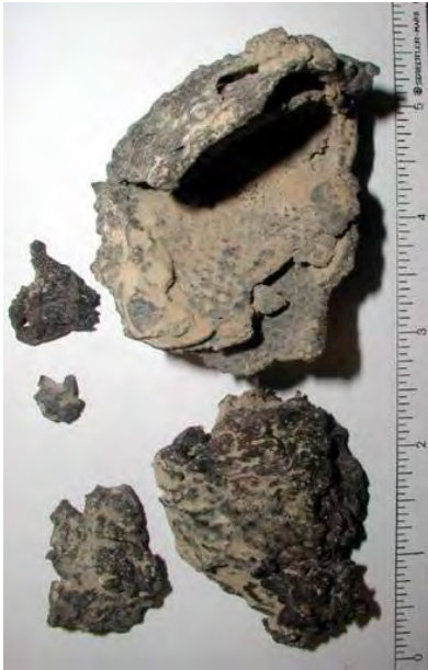
Fused Plate Catalyst After Fire Found In Downstream Ductwork
