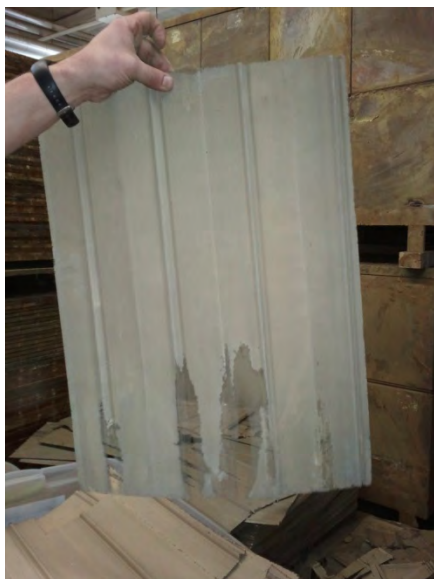
Corrosion Loss From Plate Trailing Edge
