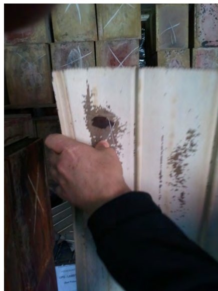
Brittle Material Breaks Out With Thumb Pressure
